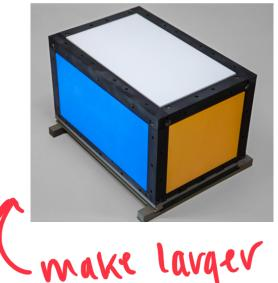
Design constraints were focused on creating the maximum surface area of colored panels, easy manual machineability in a short time frame, strong internal structure for vibration test.
