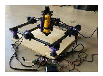
**Finished CNC assembled** with DeWalt router attached.
