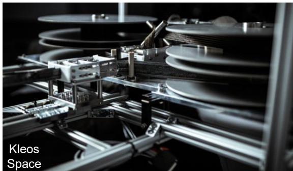
Extrusion of CF/epoxy
