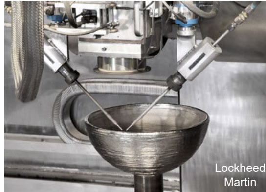
Electron beam metal additive manufacturing (EBAM)
